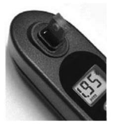
Expect the result to be within 0.15 units from previous calibration. If variation is greater, please re-check your ZERO procedure (steps 5-7) and be sure to use clean water (deionized or distilled is necessary).
