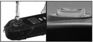
3. SELECT the test. Press the MENU button until the display shows CLH. (Chlorine Total, High)
