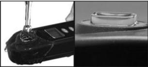
3. SELECT the test. Press the MENU button until the display shows CL. (Chlorine Free)
