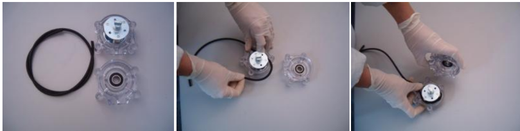
Figure 9-1: Pump tubing replacement details
