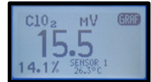
Chlorine Dioxide mV Screen
