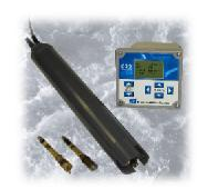
concentration equilibrium and potassium ion interference on the ammonium electrode are preformed automatically in the HYDRA C22 analyzer. The sensor uses a compressed air spray cleaner to keep the sensors clean and maintenance to a minimum. Each of the electrodes is long lived (typical 6 month life) economical and easily replaceable. Internal signal conditioners allow the sensor to be mounted hundreds of feet from the analyzer.
