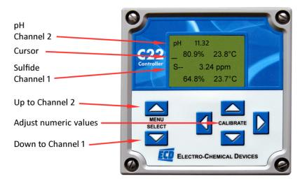
are also used to Save/Accept the calibration data and exit the calibration menu.
