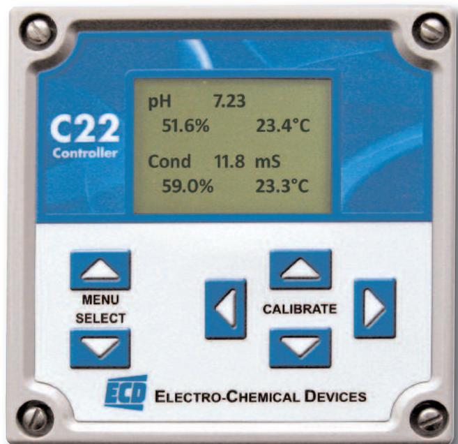
Measure pH, ORP, Specific Ion, Dissolved Oxygen, Turbidity, Chlorine, Conductivity and Resistivity with S10, S17, TR6 or various Chlorine Sensors
