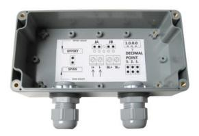
Example to re-calibrate: Meter to read 02.00pH at 4mA and 12.00pH at 20mA.
