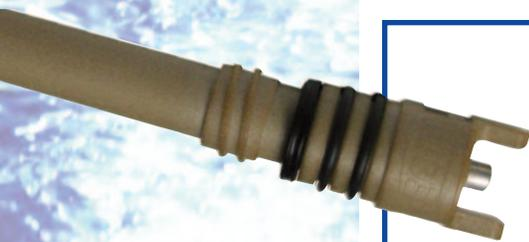
**2005167** – This **ORP (Oxidation Reduction Potential) Electrode** has a two tine PEEK body, double junction reference and a platinum tip. This general purpose sensor can be used for monitoring the oxidant level of cooling towers, swimming pools, aquariums or the de-chlorination of waste water. Metal finishing and mining also provide applications such as cyanide destruction and monitoring chrome plating baths.
