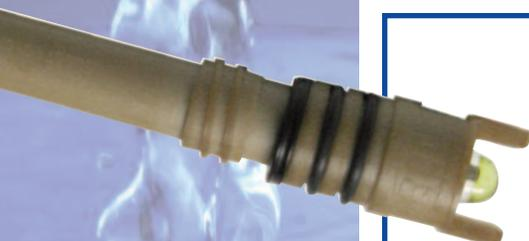
**2005157** – This **High Temperature Electrode** has a two tine PEEK body, triple junction reference and hemispherical pH bulb. This electrode is designed for the process control or neutralization of most mineral acids and bases in applications up to 130°C. The triple junction design is resistant to sulfide ion poisoning making it ideal for use in petroleum refineries and metal processing plants.
