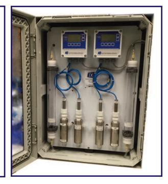
than a standard conductivity measurement. Oxygen Scavengers, such as ammmonia and amines, which give high value, are removed after the cation resin. Provide s indication measurement of impurities in the medium. The CE800 also has the option to provide pH using ECD S80 High Purity Water electrode sensor. This also provides a secondary indication of possible water contamination to do a pH change before and after the cation resin.
