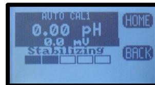
At the end of each calibration the Offset and Slope are displayed in the respective units, pH, mV, ppm, mg/l.
