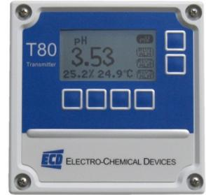
The Model T80 transmitter can be loop powered, 24 VDC powered or 100-240 VAC line powered. The standard configuration has a 4-20 mA output and a RS485 serial communication port with MODBUS® RTU output. A HART® communication version (single channel version only) is also available. Alarm relays are optionally available on either line powered transmitter.
