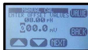
Example: MANUAL Calibration for a pH electrode
